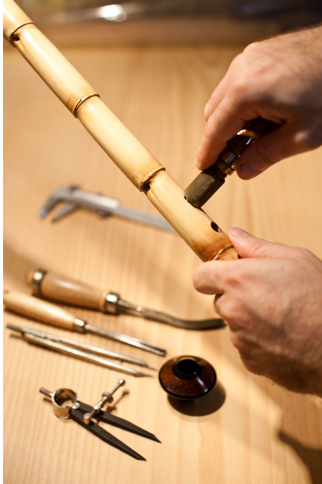
Figure 2. Opening tone holes on the reed. (© Hezarfen Ney School, reproduced with permission.)
