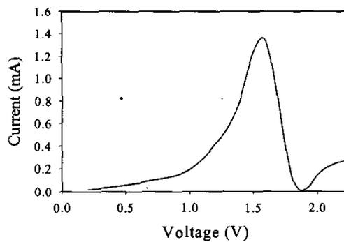
Figure 1.  $I$ - $V$  characteristics of the In<sub>0.53</sub>Ga<sub>0.47</sub>As/AlAs resonant tunneling diode.
