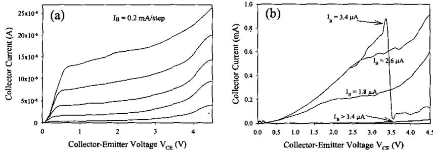
Figure 3. Common-emitter current-voltage characteristics of the RTBT with the base current of (a)  $I_B = 0.2 \mu\text{A}/\text{step}$ , (b)  $I_B = 0.8 \mu\text{A}/\text{step}$  starting from  $I_B = 1.8 \mu\text{A}$ .
