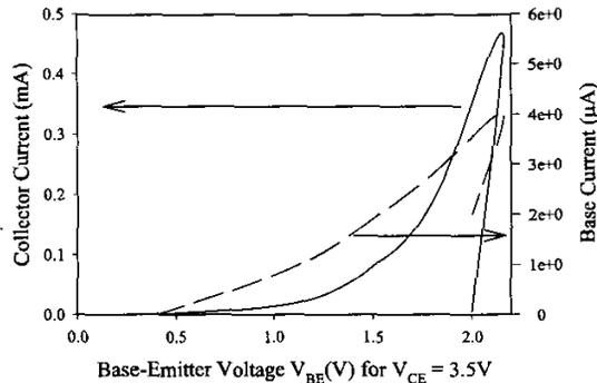
Figure 2. Common-emitter collector and base currents as functions of the base-to-emitter voltage,  $V_{BE}$ , with a constant collector-to-emitter voltage of 3.5 V.
