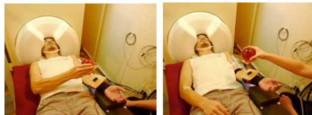
Figure 1: Subject's position in MSR during bimanual load-lifting task. During a voluntary trial, the subject lifted the 1-kg weight using the right hand ( left ). During an imposed trial, an experimenter lifted the weight unexpectedly ( right ).
