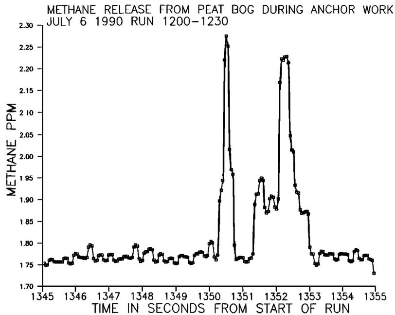
Figure 3. A methane release from the peat bog during tower anchor work.
