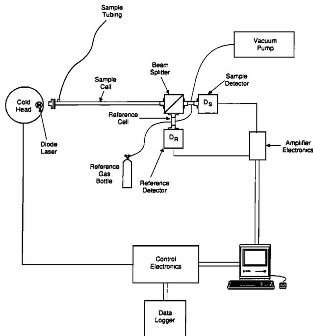
Figure 1. Tunable diode laser methane sensor schematic.
