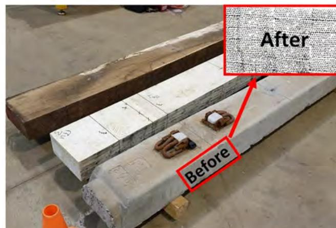
**Figure 6.** Sleeper samples showing applied speckle pattern.
