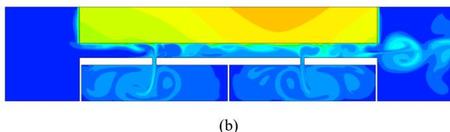
Fig. 4 Instantaneous temperature contours (xy-plane) at different instant of the 10th cycle of the in-phase oscillating case with 2 mm orifice spacing: (a)  $t^* = 10$  and (b)  $t^* = 10.5$
