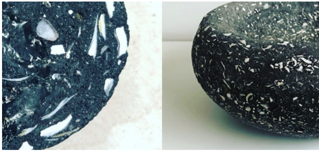
Fig. 8: Composites made of concrete and crushed oyster shells for the large-scale prototype
