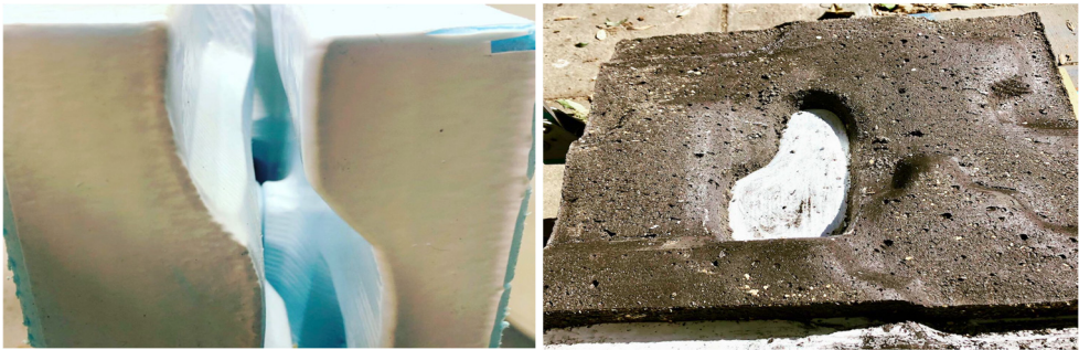
Fig. 12: CNC fabricated mould and concrete prototype to be placed into water for testing
