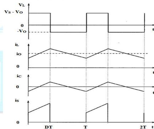
Fig. 6. Waveform for buck converter
