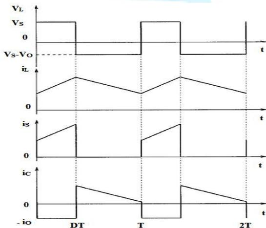
Fig. 6. Waveform for boost converter
