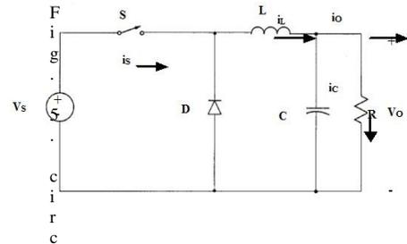
Fig.5 Circuit diagram of Buck converter
