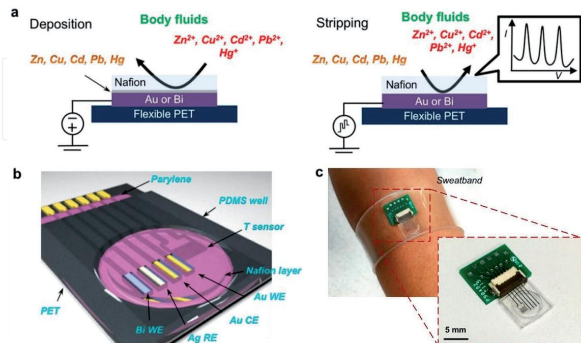
**Figure 2.** (a) A schematic showing the concept of deposition and stripping on microelectrodes. (b) A schematic showing the composition of the microsensor array. (c) Optical image of a flexible sensor array interfacing with a flexible printed circuit connector [28].
