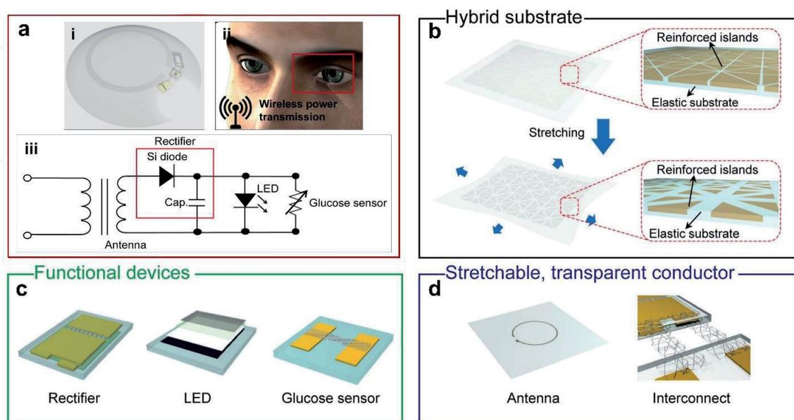
**Figure 1.** (a) (i) Schematic illustration and (ii) operation of the soft, smart contact lens and (iii) the circuit diagram of the smart contact lens system. The soft, smart contact lens is composed of (b) a hybrid substrate; (c) functional devices including rectifier, LED, and glucose sensor; and (d) a transparent, stretchable conductor for antenna and interconnects [17].
