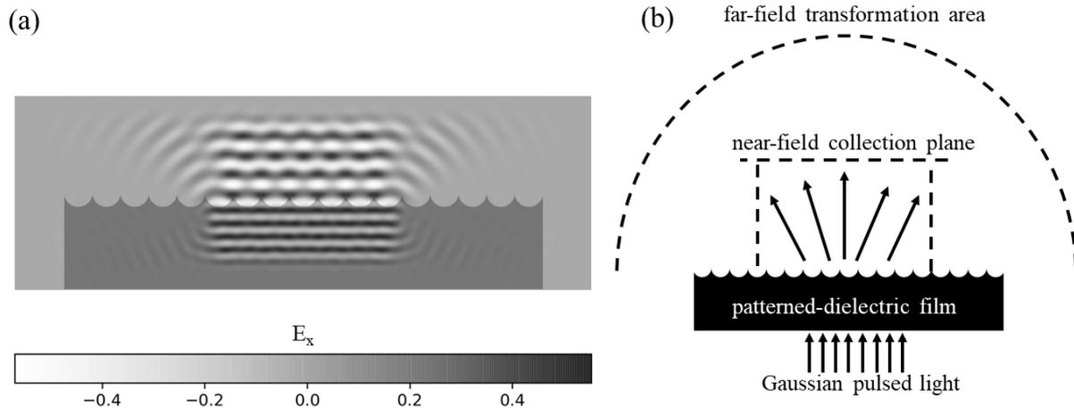
**Figure 1.** (a) computed model of dielectric film with curvature hole shown in  $E_x$  field and (b) diagram of far-field transformation from near-field collection plane.
