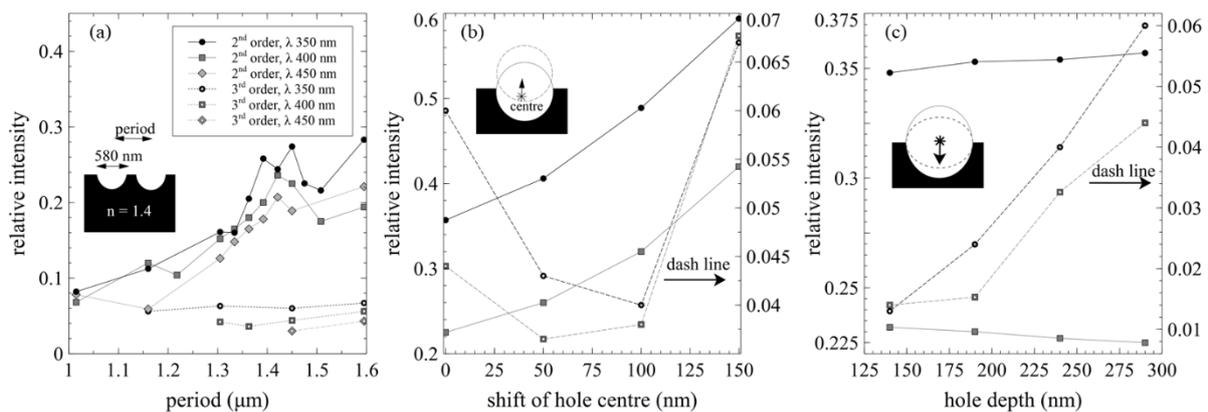
**Figure 2.** Relative intensities of the second diffraction order to the first and the third order to the first affected by (a) period change, (b) shifted centre of hole and (c) depth of hole shown in wavelengths of 350 nm, 400 nm and 450 nm.
