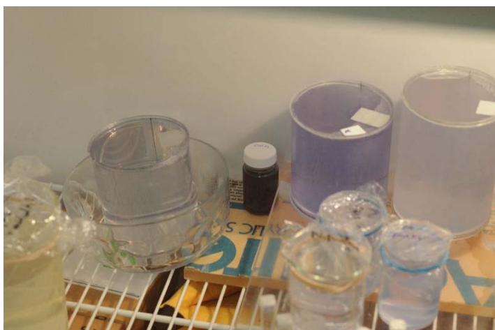
Figure 6. Photograph inside storage refrigerator of three 10 cm diameter gels, same formula but different batches, demonstrating marked changes in initial colour and scatter.
