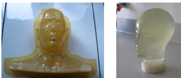
Figure 2. Antropomorphic shaped Barex phantom (a) and glass phantom (b) filled with polymer gel.
