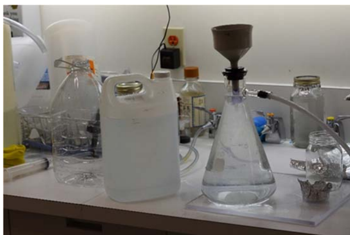
Figure 4. Photograph of vacuum filter and flask, filtering refractive index optimization solution of propylene glycol and water.
