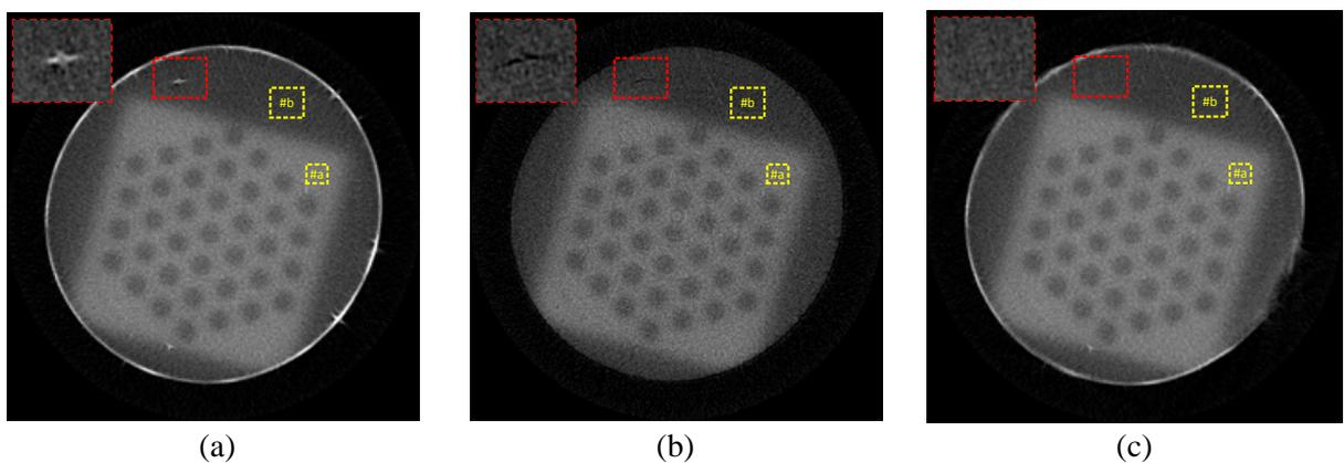
**Figure 4.** Reconstructed images of different methods: (a) mono-wavelength, (b) dual-wavelength via Equation (1) and (c) proposed method. The red box depicts the zoomed ROI with a dust stain visible in (a), replaced by a *negative scar* in (b), and clearly removed in (c). The yellow boxes ROI #a and ROI #b are selected to calculate the SNR and CNR.
