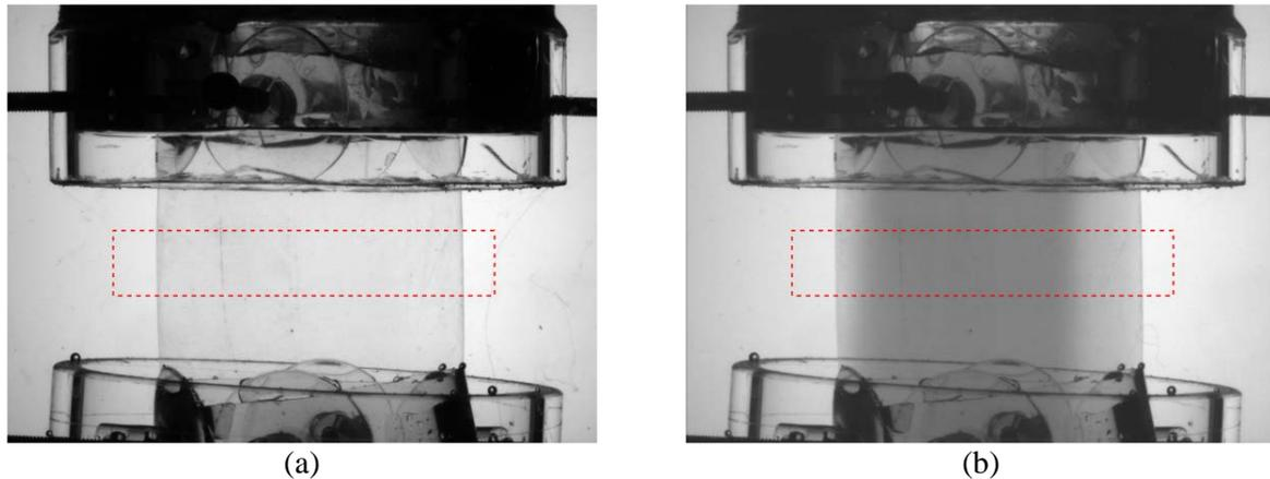
**Figure 2.** Reference (a) and data (b) projection scans of the silicone dosimeter (FlexyDos3D) phantom. The red box depicts the ROI for following data processing.
