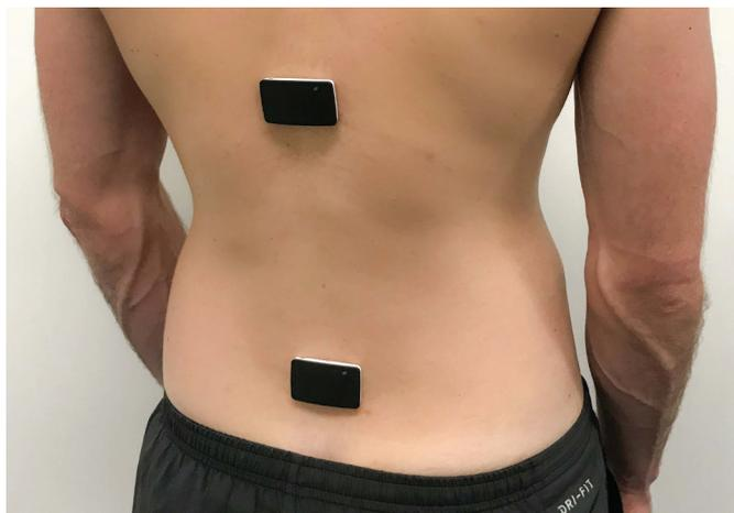
Hypoallergenic over-wraps are applied when used during normal daily activities. When EMG sensors are included, they are placed paraspinally at the L3 level.
